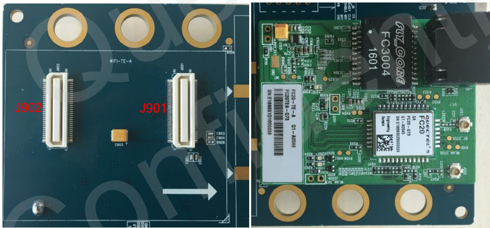
Figure 10: Connection Between FC20 TE-A and EVB
