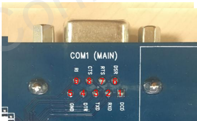
Figure 25: Pin Assignments of J401
